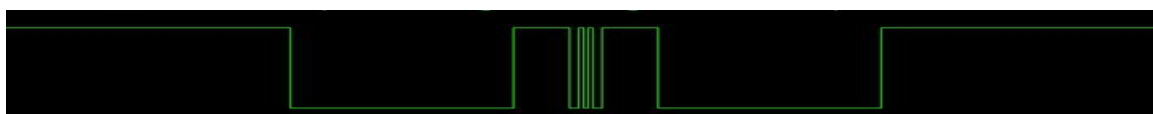
Image 2: A single MIBAM pulse waveform. Each bit has a specified weight (period of time), and the channel's output is high if that bit is a binary '1'. Notice that the two halves form a mirror image of one another.
