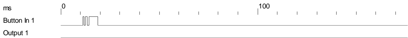
Figure Four: Signals Shorter Than 25ms Will Not Trigger an Output Pulse
