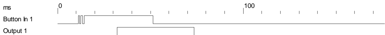
Figure Two: A Single Button Press and the Corresponding EDE2008 Debounced Output
